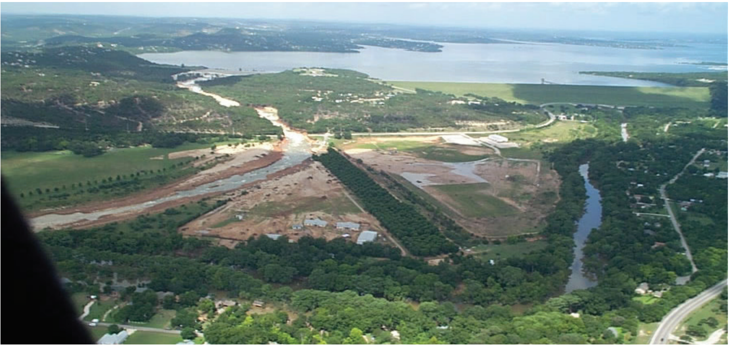
Figure 9. Emergency spillway in use at Canyon Lake July 2002.
