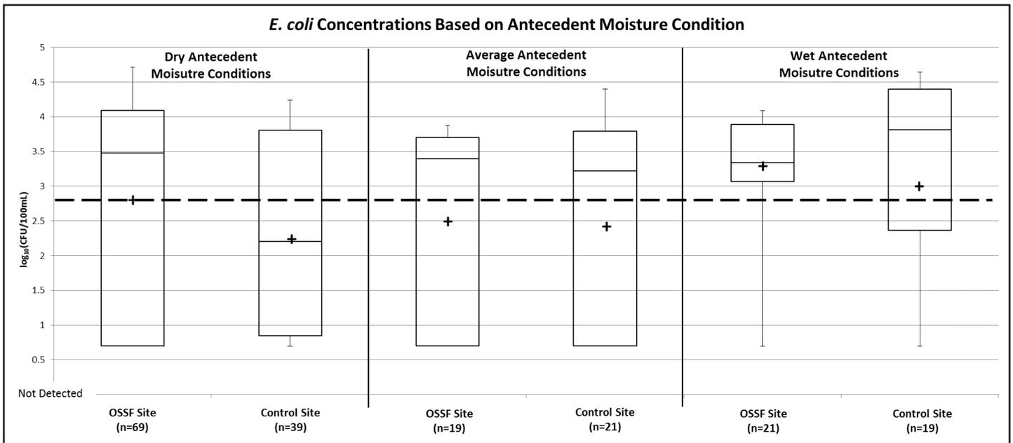
**Figure 3.** Quartile plots of *E. coli* concentrations found in runoff at the 2 monitoring sites in the Dickinson Bayou watershed separated by antecedent moisture conditions. The plus symbol represents the mean value of each of the 2 datasets. The dashed line represents the Texas state recreational contact standard for *E. coli*.
