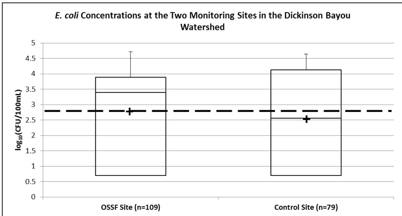
**Figure 2.** Cumulative distribution plots of *E. coli* concentrations found in runoff at the 2 monitoring sites in the Dickinson Bayou watershed. The dashed line represents the Texas state recreational contact standard for *E. coli*.
