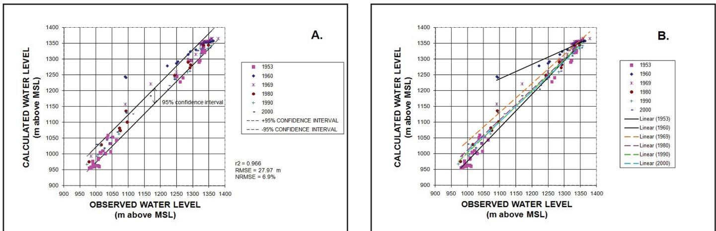
**Figure 6.** Calibration results for the exploitation period showing correlation between observed and calculated water levels.
