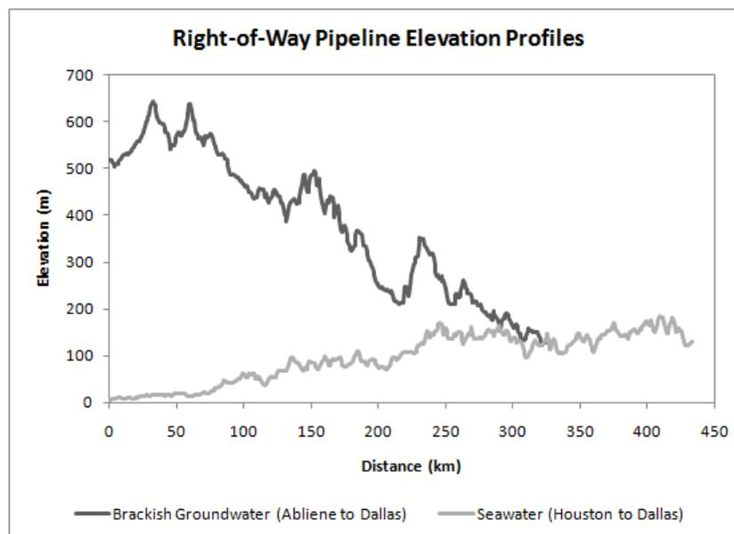
**Fig. 7.** Elevation profiles for the seawater and brackish groundwater pipelines show a general uphill route for seawater and downhill route for brackish groundwater. Despite these trends, elevation increases along the brackish groundwater pipeline are larger than those increases of the seawater pipeline.
