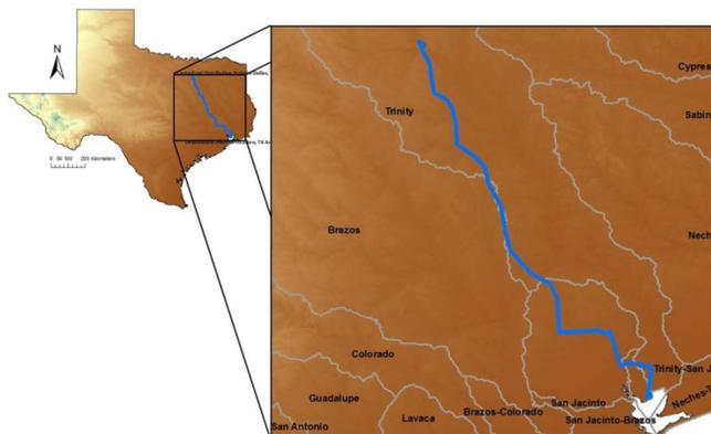
**Fig. 5.** The seawater right-of-way long-haul transfer pipeline passes back and forth between major river basins: Trinity-San Jacinto, Trinity, San Jacinto, and Brazos, before ending in the Trinity basin.
