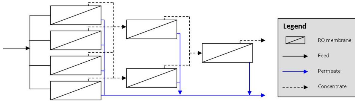
**Fig. 1.** Typical reverse osmosis units are configured in a cascade layout to improve water recovery, which typically ranges from 35% to 50% for seawater and 60% to 85% for brackish groundwater (Lawler and Benjamin 2008; Zander et al. 2008).
