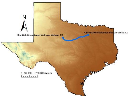
**Fig. 4.** An alternative desalination and long-haul transfer water supply for Dallas analyzed here is brackish groundwater desalination near Abilene with a long-haul pipeline following existing road right-of-ways.
