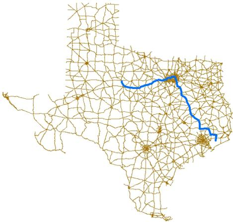
**Fig. 2.** Major Texas roads and highways were used to determine the right-of-way long-haul pipeline routes such that the routes follow existing easements. The brackish groundwater pipeline is shown traveling west to east and the seawater pipeline is shown traveling southeast to northwest.
